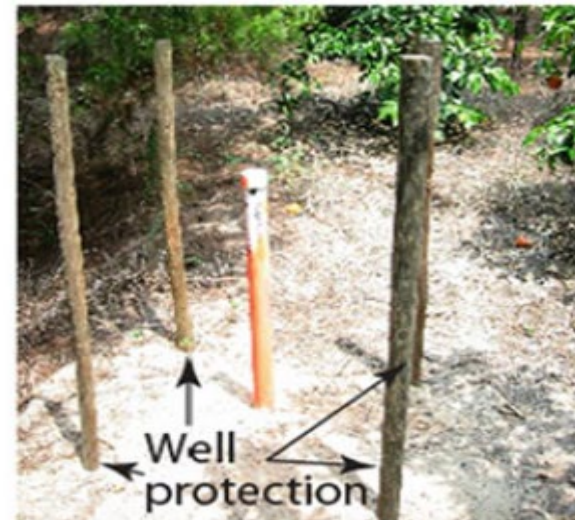
Fig. 3.41 Typical installation to quantify horizontal and vertical hydraulic gradient, seepage rate, and hydraulic conductivity
