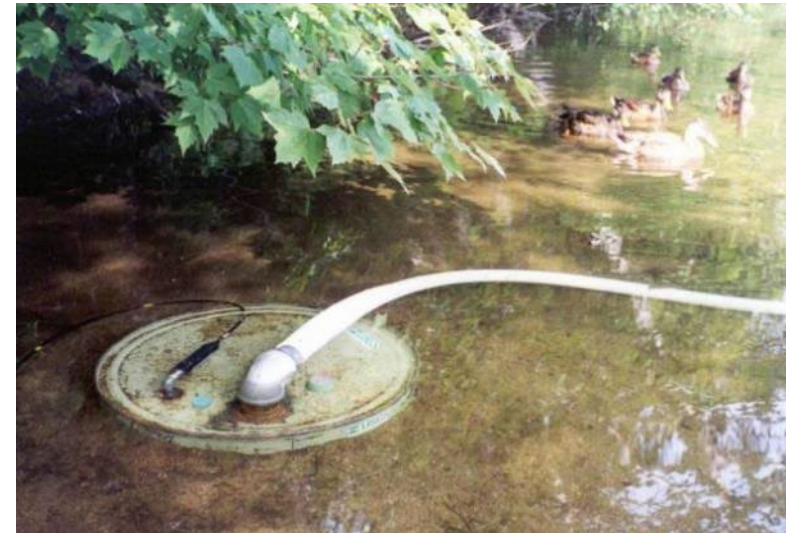
Electromagnetic seepage meter
